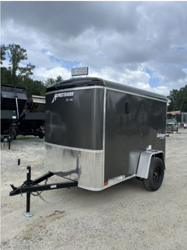
2026 Homesteader Trailer / Challenger Series / 5x8 / 5'7" Interior Height / Single Swing Rear Door / 32" Side Door / 24" Stoneguard / .030 Charcoal Gray Aluminum
