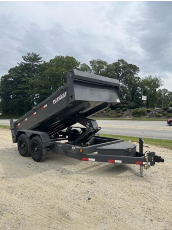
2027 Norstar DCB Series / 72" X 12' / 2-5,200# Electric Brake Axles / Scissor Hoist / Barn Door Rear Gates / Ramps
