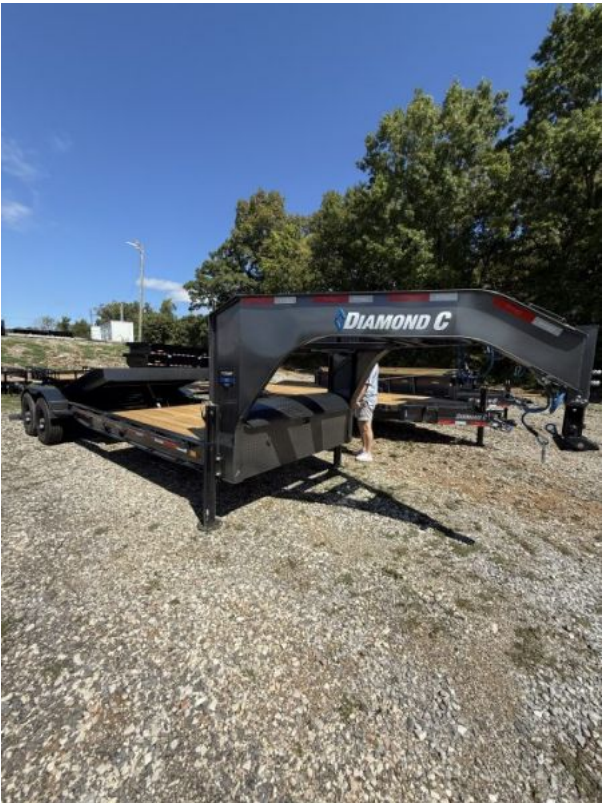
2027 Diamond C HDT 210 24' Tilt Trailer, PACESETTER EDITION, HYD JACKS, FORK HOLDERS, 23K GVWR, ABS BRAKES
